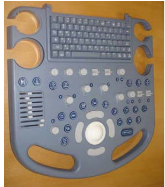
Figure 8-53 Unscrewing 9 screws and lifting up the MAIN OPIO
