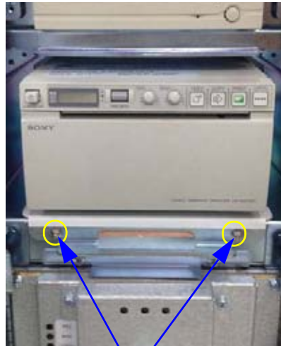
Assemble printer base plate with two screws
