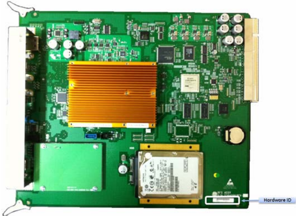
Figure 8-75 Hardware ID on label RFS-board
