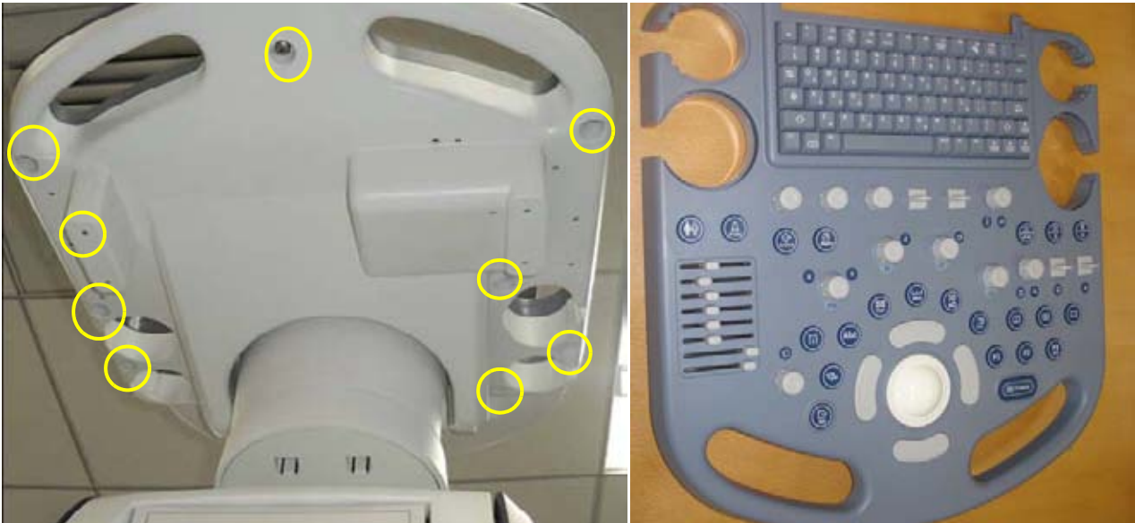
Figure 8-26 Separating the MAIN OPIO
