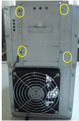
Figure 8-90 Opening the rear bracket
