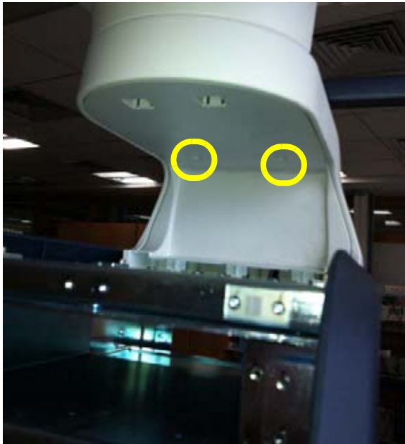
Figure 8-66 Remove REAR COVER ASSY
