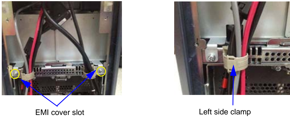
Figure 8-114 Route the printer cables
