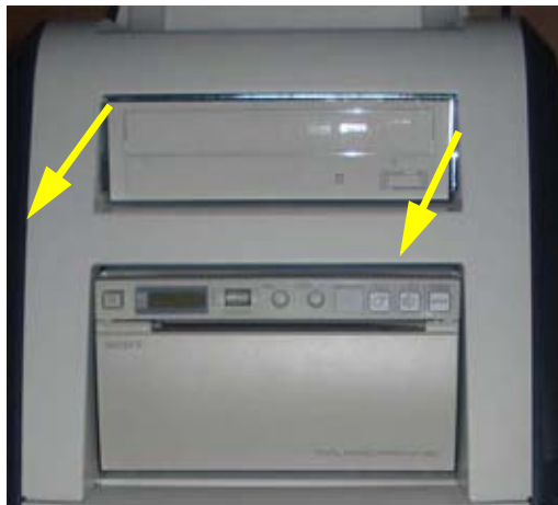
Figure 8-94 Removing FRONT PLASTIC COVER
