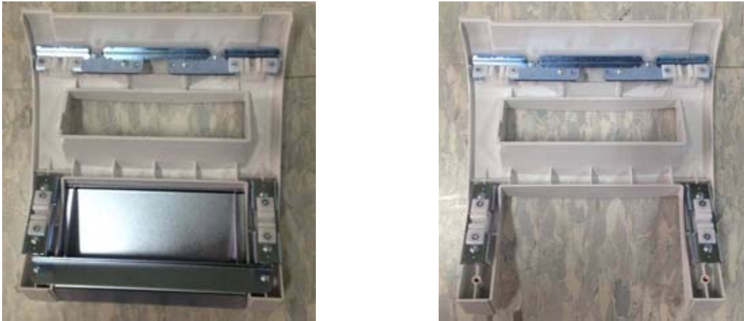
Figure 8-106 Disassemble printer cover
