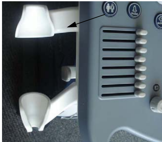
Figure 8-130 HORIZONTAL TV PROBE HOLDER is installed on Left Side only
