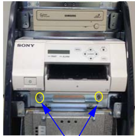
2 screws (2159634 -screw BH M4X10)
