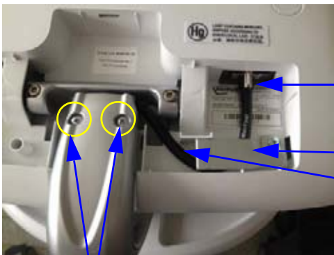
Unscrew the fastener
