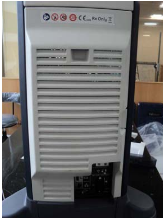
Figure 8-33 Unscrewing 5 screws and Remove REAR COVER ASSY
