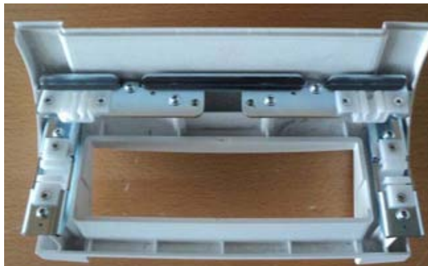
Figure 8-126 Assemble DVD front cover
