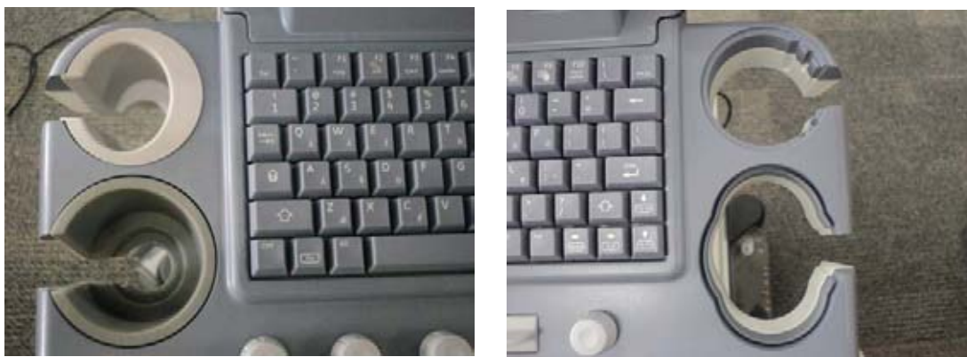
Figure 8-25 Removing the 4 PROBE HOLDERS
