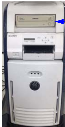
Figure 8-128 Assemble the front cover
