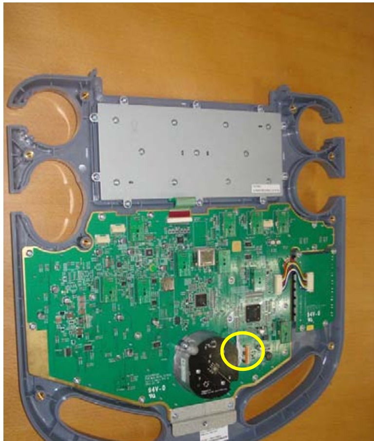
Figure 8-55 Disconnecting the TRACKBALL CABLE
