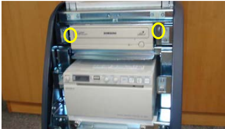
Figure 8-96 Removing the DVD
