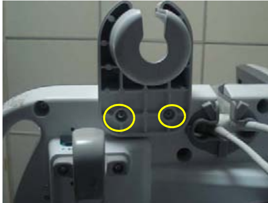
Figure 8-131 Assemble TV PROBE HOLDER BASE with 2 screws (2159634, BH M4x10)
