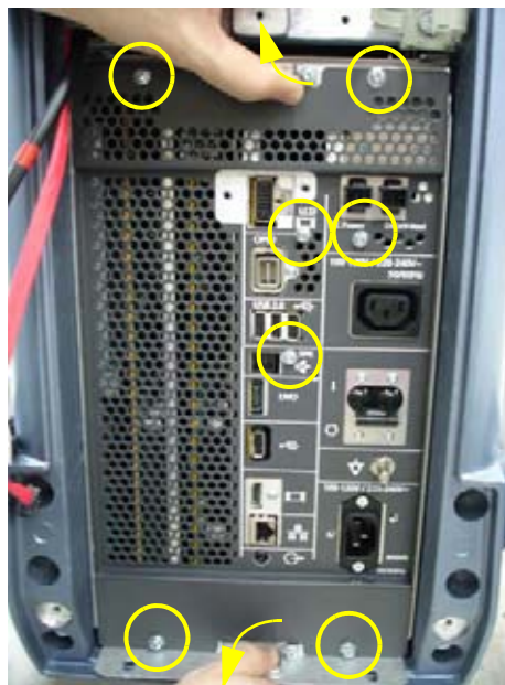
Figure 8-43 Pulling out the NEST
