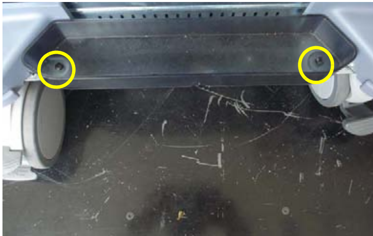
Figure 8-65 Unscrewing 2 screws and remove SIDE TRAY ASSY
