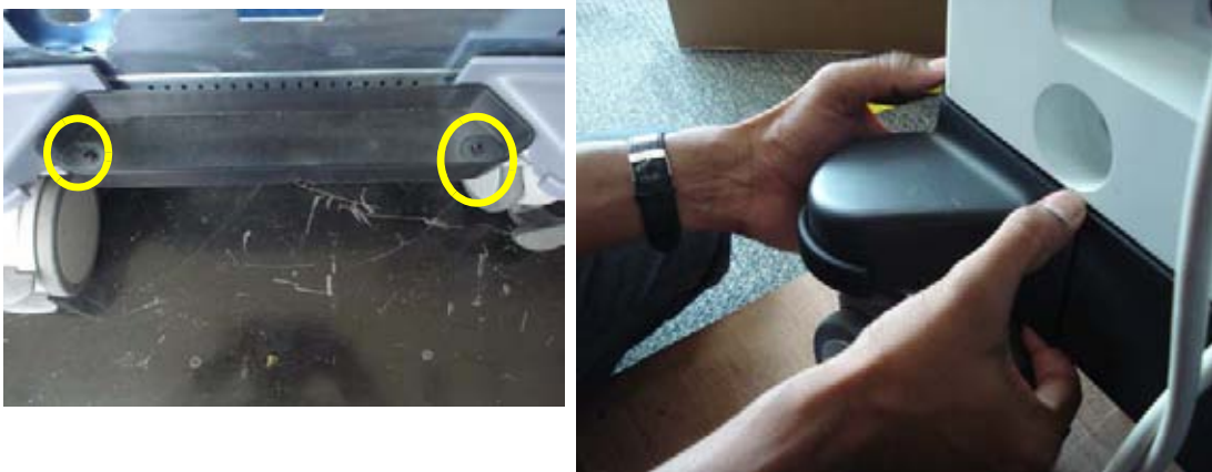
Figure 8-62 Removing the CASTER CAP
