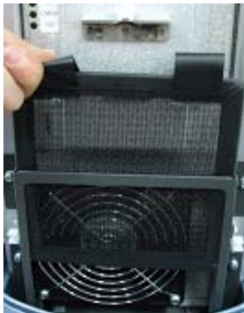
Figure 8-45 Removing the AIR FILTER
