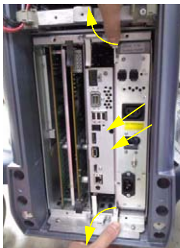
Figure 8-71 Drawing the CPS
