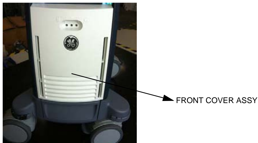
Figure 8-50 Removing the FRONT COVER ASSY
