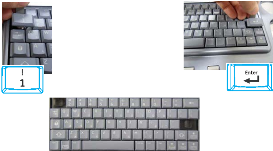
Figure 8-99 removing “1” key and “Enter” key
