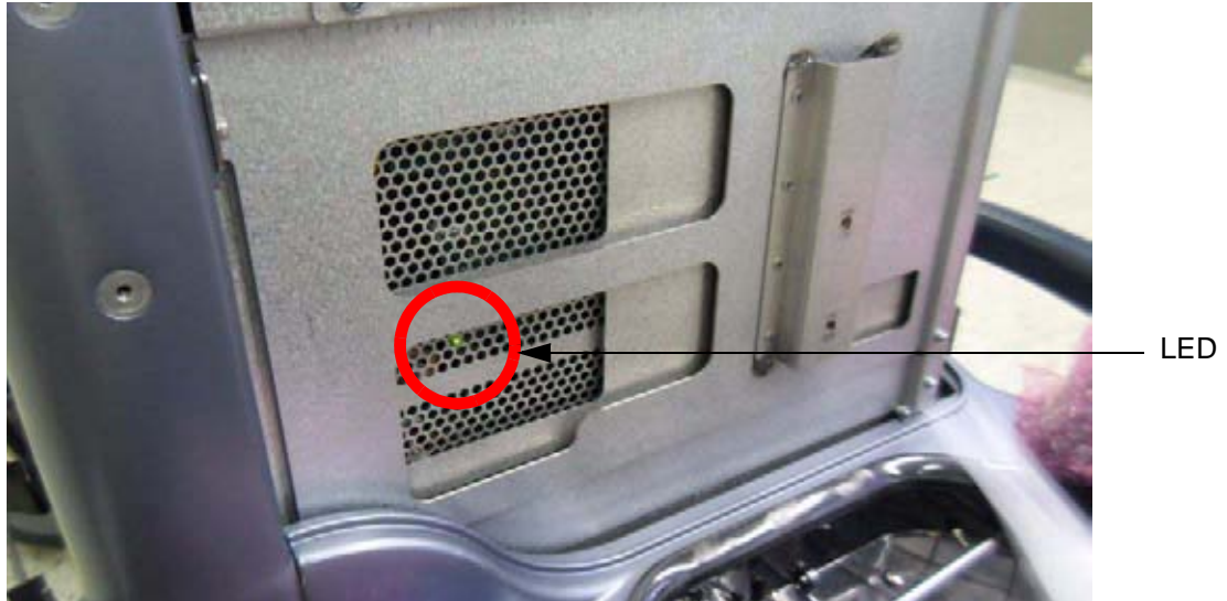
Figure 7-6 Check green LED inside CPS
