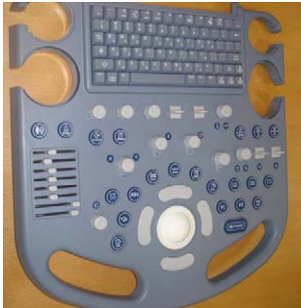
Figure 8-57 Removing 8 TGC KNOBS
