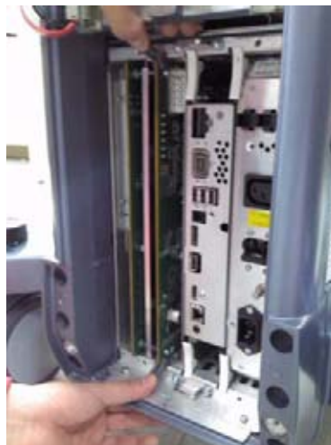
Figure 8-87 Drawing the BF/PIR
