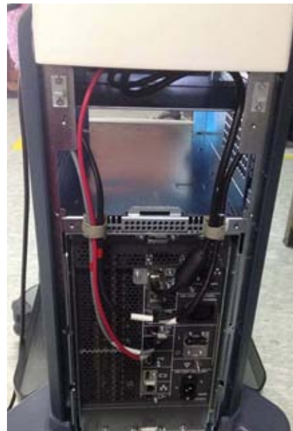
Rear side view after removing the EMI covers 1 and 2
