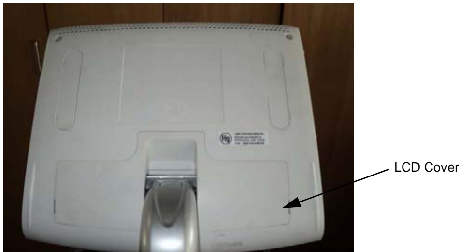
Figure 8-22 Removing the LCD COVER
