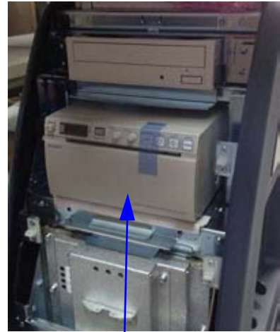
Push the printer assembly
