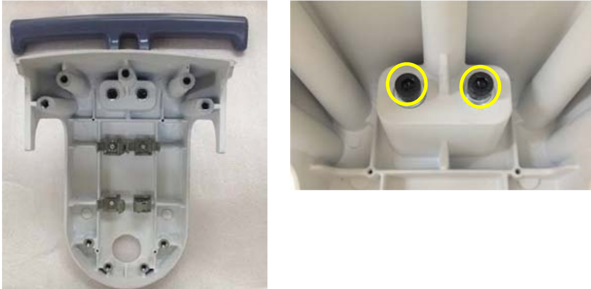
Figure 8-67 Unscrewing 2 screws and remove REAR HANDLE
