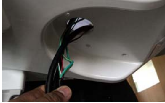
Lift the base and pull the LCD cable, OPIO cable and Speaker cables through the keyboard base hole
