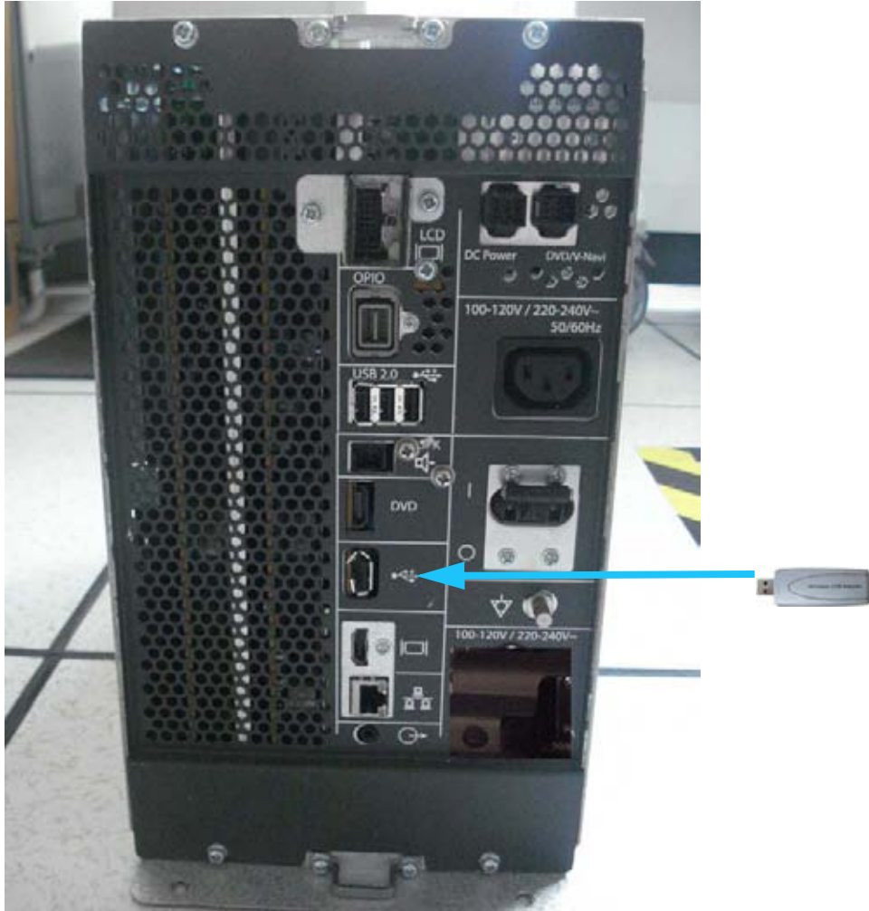
Figure 3-9 Connection Scheme - Wireless (USB) Network Adapter
