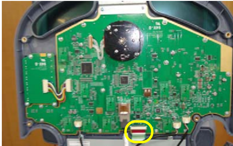
Figure 8-101 Disconnecting 3 cables from OPIO ASSY
